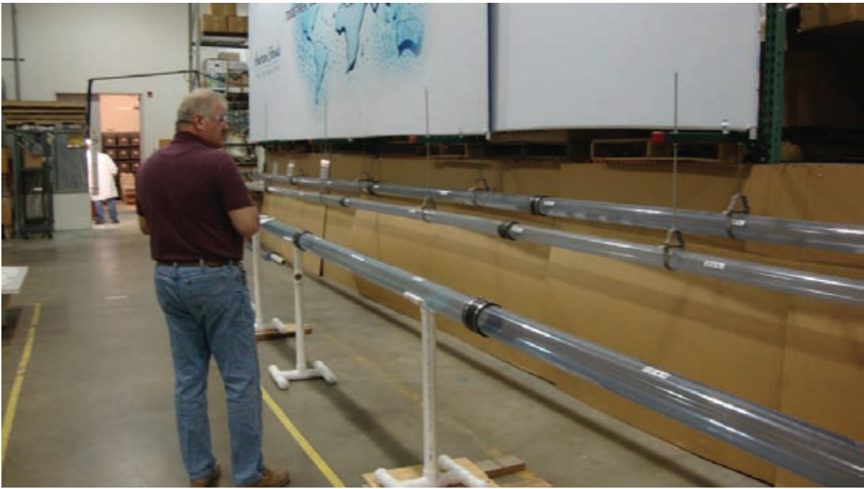
PHOTO 5-C LEAD TECHNICIAN RECORDING TEST MEDIA TRAVEL DISTANCES
