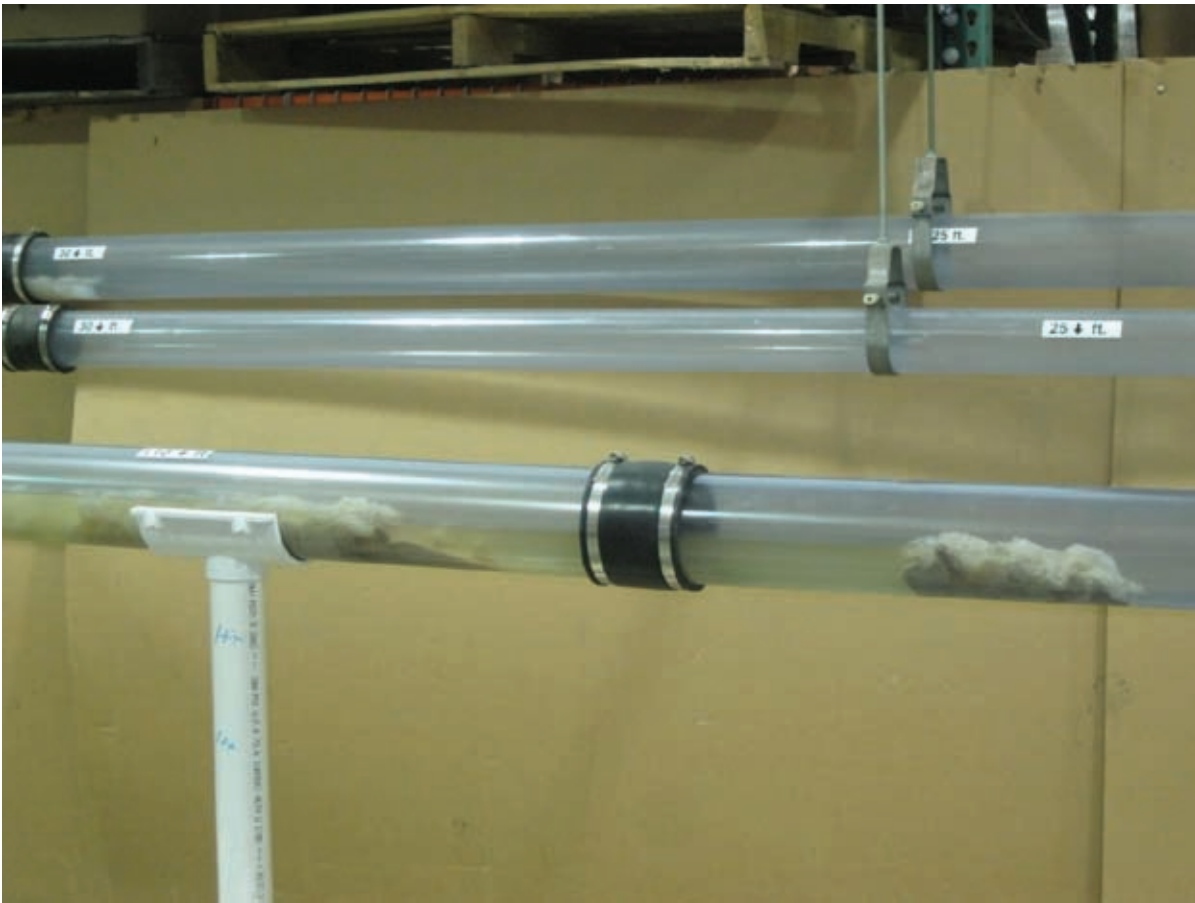
PHOTO 7-E ORDERLY FLOW OF SOLIDS IN TEST RUN #3 @ 1.28 GALLON (4.8 L) VOLUME, 1% SLOPE
